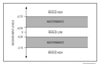
Figure 4a. Receiver Positive/Negative Thresholds for INVALID
