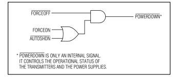
Figure 3d. Power-Down Logic
