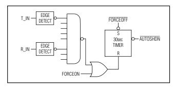
Figure 3c. AutoShutdown Plus Logic
