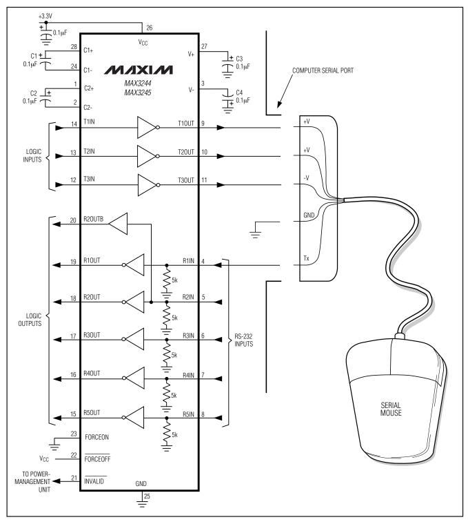
Figure 11b. Mouse Driver Test Circuit
