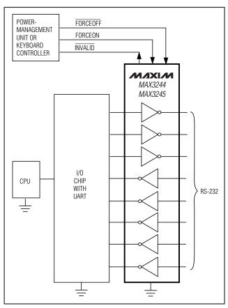
Figure 1. Interface Under Control of PMU
