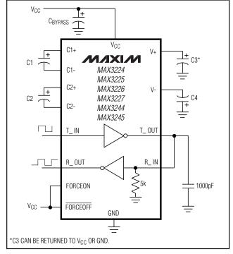
Figure 7. Loopback Test Circuit
