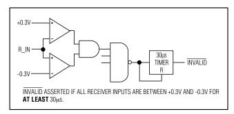
Figure 3a. INVALID Functional Diagram, INVALID Low
