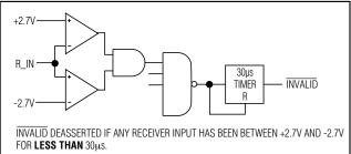
Figure 3b. INVALID Functional Diagram, INVALID High
